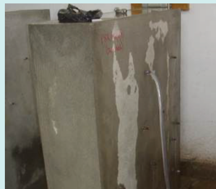
Fig-22d: Watering of the Specimen through Nozzles
