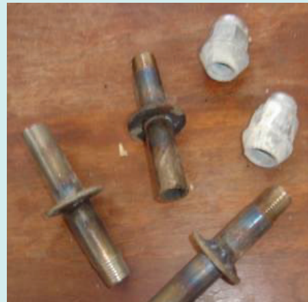
Fig-22a. Injection Nozzles and Stoppers
