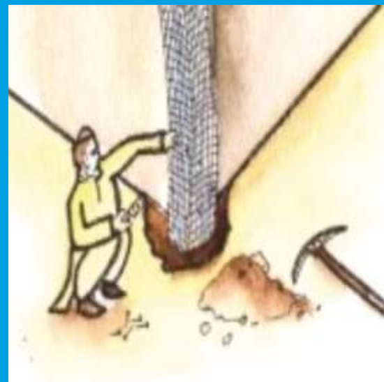
Anchoring vertical belt 300 mm below plinth level
