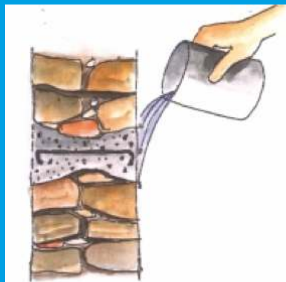
Water curing for 10 days
